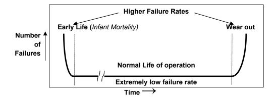
**Infant Mortality Screening (During Production).** Normal production devices are baked for minimum of 96 hours at 170°C to screen out failures attributed to random defects. For other than data retention mechanisms, burn-In of units for 168 hours @125°C (Mil-Std-883B) is recommended.
