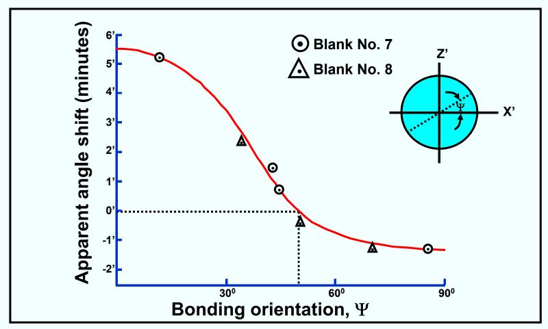
When 22 MHz fundamental mode AT-cut resonators were reprocessed so as to vary the bonding orientations, the frequency vs. temperature characteristics of the resonators changed as if the angles of cut had been changed. The resonator blanks were 6.4 mm in diameter plano-plano, and were bonded to low-stress mounting clips by nickel electrobonding.
