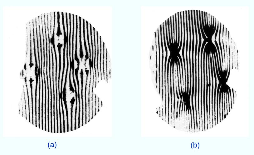
X-ray topographs showing lattice distortions caused by bonding cements; (a) Bakelite cement - expanded upon curing, (b) DuPont 5504 cement - shrank upon curing
