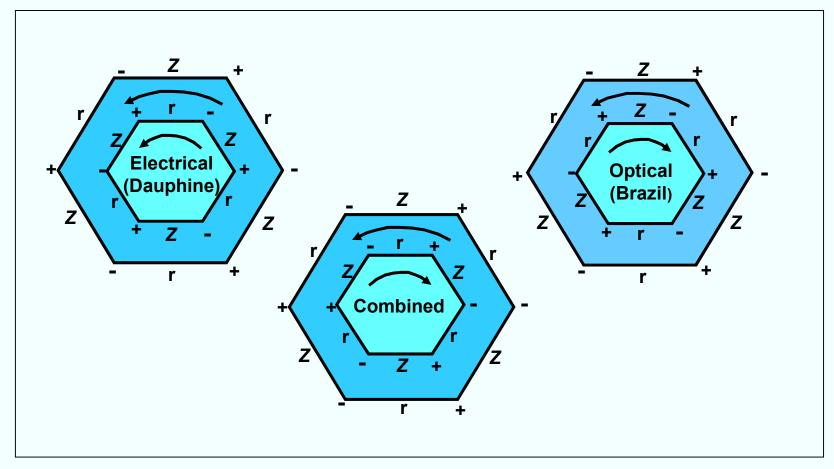
The diagrams illustrate the relationship between the axial system and hand of twinned crystals. The arrows indicate the hand.
