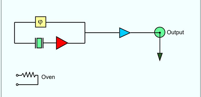
Each of the three main parts of an OCXO, i.e., the crystal, the sustaining circuit, and the oven, contribute to instabilities. The various instabilities are discussed in the rest of chapter 3 and in chapter 4.
