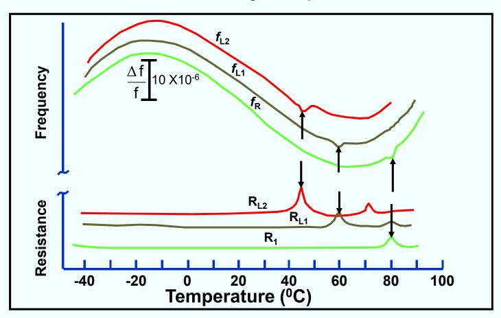
Activity dips in the f vs. T and R vs. T when operated with and without load capacitors. Dip temperatures are a function of  $C_L$ , which indicates that the dip is caused by a mode (probably flexure) with a large negative temperature coefficient.
