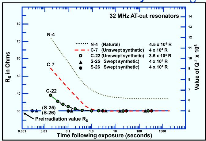
The curves show the series resonance resistance,  $R_s$ , vs. time following a 4 x 10<sup>4</sup> rad pulse. Resonators made of swept quartz show no change in  $R_s$  from the earliest measurement time (1 ms) after exposure, at room temperature. Large increases in  $R_s$  (i.e., large decrease in the Q) will stop the oscillation.
