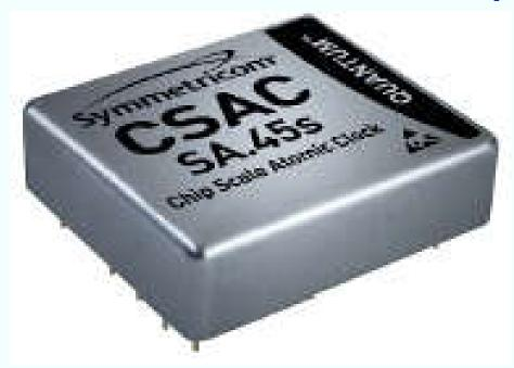
120mW power consumption 16cm<sup>3</sup> volume (1.6" x 1.39" x 0.45") 35g weight
