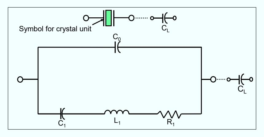
$$\frac{\Delta f}{f_{\text{S}}} \approx \frac{C_{\text{1}}}{2(C_{\text{0}} + C_{\text{L}})} \rightarrow \begin{cases} \text{1. Voltage control (VCXO)} \\ \text{2. Temperature compensation} \\ \text{(TCXO)} \end{cases}$$
