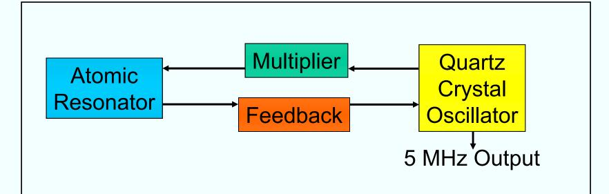
Let the servo loop time constant =  $t_0$ , let the atomic standard's  $\Gamma = \Gamma_A$ , and the crystal oscillator's (VCXO's)  $\Gamma = \Gamma_O$ . Then,
