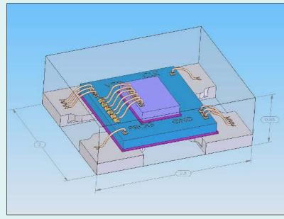
Resonator (Si): 0.2 x 0.2 x 0.01 mm<sup>3</sup> 5 MHz; f vs. T: -30 ppm/°C
