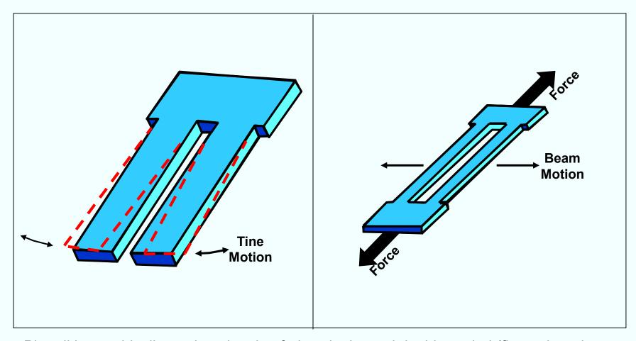
Photolithographically produced tuning forks, single- and double-ended (flexural-mode or torsional-mode), can provide low-cost, high-resolution sensors for measuring temperature, pressure, force, and acceleration. Shown are flexural-mode tuning forks.
