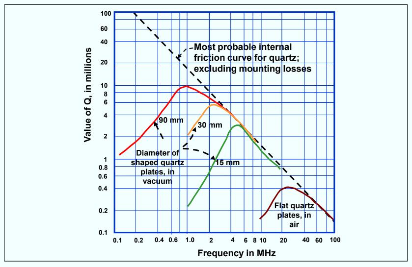
Empirically determined Q vs. frequency curves indicate that the maximum achievable Q times the frequency is a constant, e.g., 16 million for AT-cut resonators, when f is in MHz.
