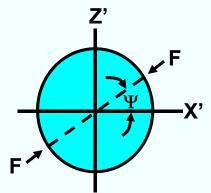
As an example, consider a 5 MHz 3rd overtone, 14 mm diameter resonator. Assuming the presence of diametrical forces only, (1 gram =  $9.81 \times 10^{-3}$  newtons),
