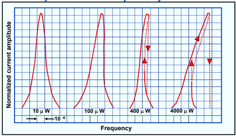
At high drive levels, resonance curves become asymmetric due to the nonlinearities of quartz.
