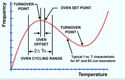
Oven Parameters vs. Stability for SC-cut Oscillator Assuming  $T_i - T_{LTP} = 10^{\circ}C$
