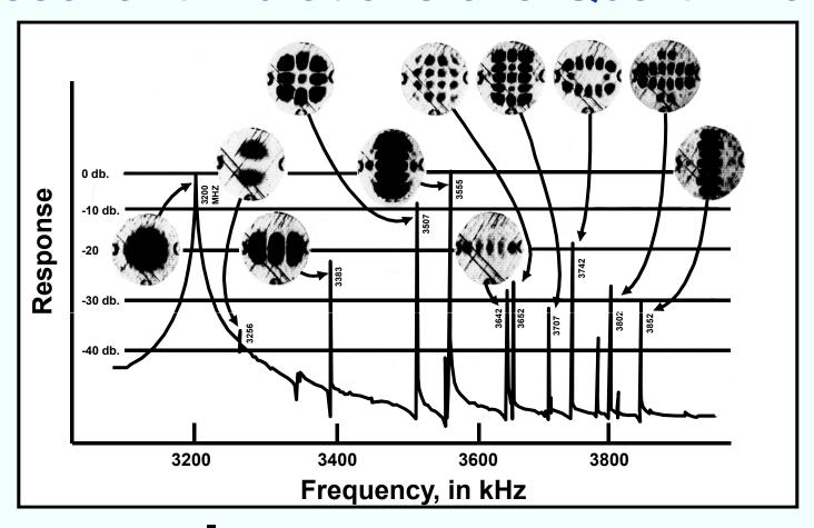
X-ray topographs (21•0 plane) of various modes excited during a frequency scan of a fundamental mode, circular, AT-cut resonator. The first peak, at 3.2 MHz, is the main mode; all others are unwanted modes. Dark areas correspond to high amplitudes of displacement.
