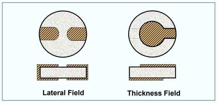
In lateral field resonators (LFR): 1. the electrodes are absent from the regions of greatest motion, and 2. varying the orientation of the gap between the electrodes varies certain important resonator properties. LFRs can also be made with electrodes on only one major face. Advantages of LFR are:
