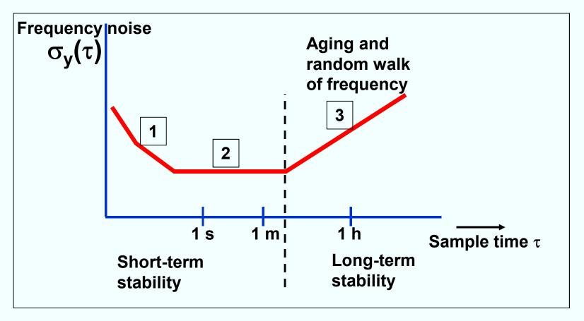
In **region 1**, the white noise region, additional averaging (more data) improves the limit of detection. In **region 2**, flicker noise, it does not. In **region 3**, it makes it worse. For  $\sigma_y(\tau)$  to be a proper measure of random frequency fluctuations, aging must be properly subtracted from the data at long  $\tau$ 's.
