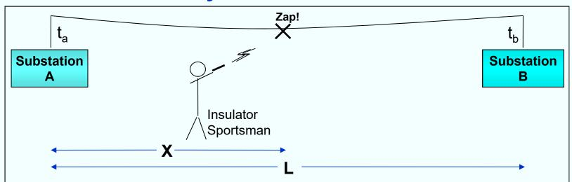
When a fault occurs, e.g., when a "sportsman" shoots out an insulator, a disturbance propagates down the line. The location of the fault can be determined from the differences in the times of arrival at the nearest substations:
