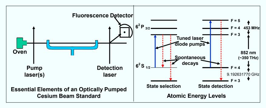
The proper atomic energy levels are populated by optical pumping with a laser diode. This method provides superior utilization of Cs atoms, and provides the potential advantages of: higher S/N, longer life, lower weight, and the possibility of trading off size for accuracy. A miniature Cs standard of 1 x 10<sup>-11</sup> accuracy, and <<1 liter volume, i.e., about 100x higher accuracy than a Rb standard, in a smaller volume (but not necessarily the same shape factor) seems possible.
