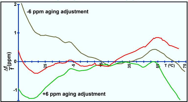
In TCXO's, temperature sensitive reactances are used to compensate for f vs. T variations. A variable reactance is also used to compensate for TCXO aging. The effect of the adjustment for aging on f vs. T stability is the "trim effect". Curves show f vs. T stability of a "0.5 ppm TCXO," at zero trim and at  $\pm 6$  ppm trim. (Curves have been vertically displaced for clarity.)
