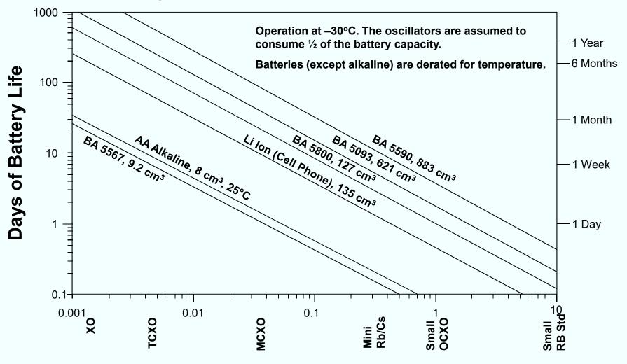
**Oscillator Power (Watts)**
