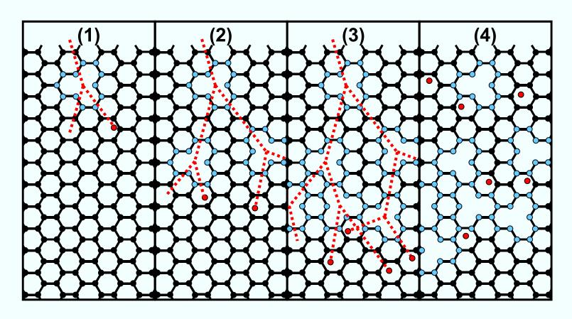
A fast neutron can displace about 50 to 100 atoms before it comes to rest. Most of the damage is done by the recoiling atoms. Net result is that each neutron can cause numerous vacancies and interstitials.
