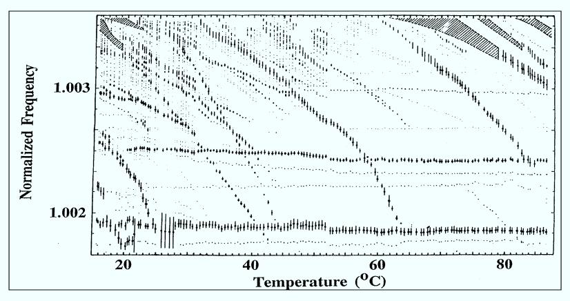
Activity dips occur where the f vs. T curves of unwanted modes intersect the f vs. T curve of the wanted mode. Such activity dips are highly sensitive to drive level and load reactance.
