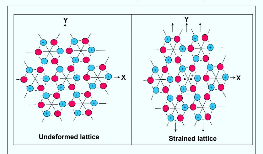
The piezoelectric effect provides a coupling between the mechanical properties of a piezoelectric crystal and an electrical circuit.
