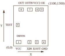
Special instruction: Keep bonding for Xin and Xout as close to die cavity edge as possible as we will mount additional 0201 component in red oval area.
