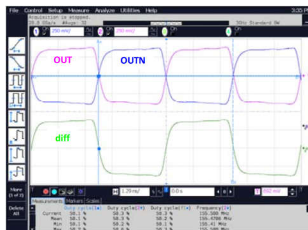
7051N1 V_{DD}=3.3V , f_0=155.52MHz , T_a=25^\circ C
