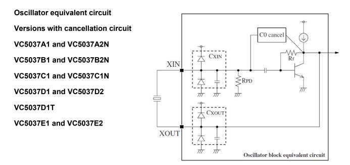
The VC5037 series oscillator circuit listed above have a C0 cancellation circuit built-in to improve the oscillator margins. If power is applied when there is an open circuit between XIN and XOUT, self oscillation (at approx 80MHz) may occur, which is not abnormal. Users should confirm that the oscillator operates normally when a crystal unit is connected. Note: Abnormally high crystal resistance may also result in self-oscillation.
