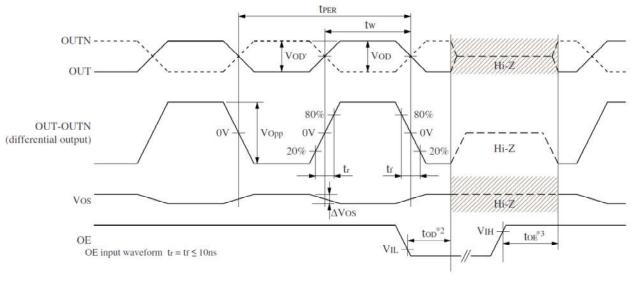
$$\begin{split} DUTY = t_W / t_{PER} \times 100 ~(\%) @ \mbox{ crossing point} \\ \Delta V_{OD} = |V_{OD}' - V_{OD}| \end{split}$$
