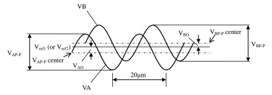
$V_{AO}$  and  $V_{BO}$  indicate the difference between the VA and VB center line and  $V_{ref1}$  (or  $V_{ref2}$ ), respectively.
