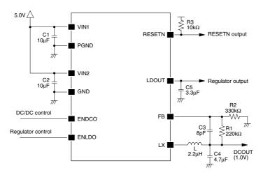
Note. RESETN is open-drain, therefore, please take care so that the High level signal does not exceed the absolute maximum rating of IC which receives the reset signal. Besides, if the rest signal is not used, RESETN should be connected to GND.
