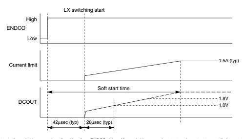
The LX starts the switching operation after  $42\mu s$  from ENDCO rising. After switching operation startup, the output current limit operates like linear increase (load current = 0A). The DC/DC converter output voltage rise time varies with the load current, output capacitance, and other conditions.
