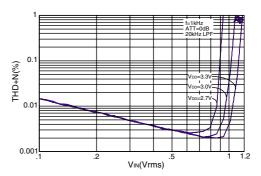
Figure 7. THD+N vs. input amplitude (SM6451A)
