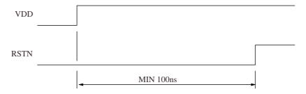
Figure 6. Reset timing
