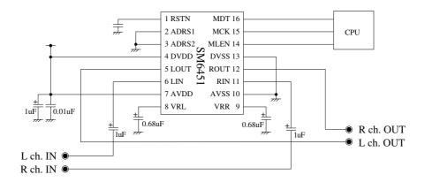
Figure 4. Typical application circuit 2
