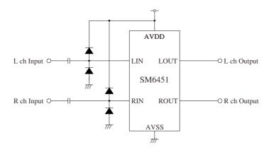
Figure 3. Input protection diodes
