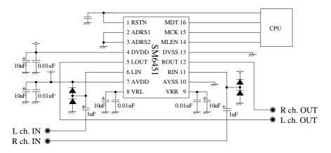
Figure 1. Typical application circuit 1
