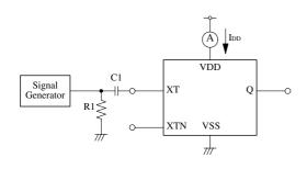
2.0Vp-p, 70MHz sine wave input signal (3V operation) 3.5Vp-p, 70MHz sine wave input signal (5V operation) C1:  $0.001\mu F$
