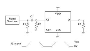
2.0Vp-p, 10MHz sine wave input signal (3V operation) 3.5Vp-p, 10MHz sine wave input signal (5V operation)
