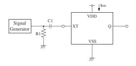
2.0Vp-p, 30MHz sine wave input signal (3V operation) 3.5Vp-p, 30MHz sine wave input signal (5V operation)
