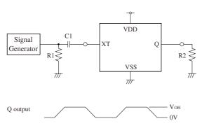
2.0Vp-p, 10MHz sine wave input signal (3V operation)
