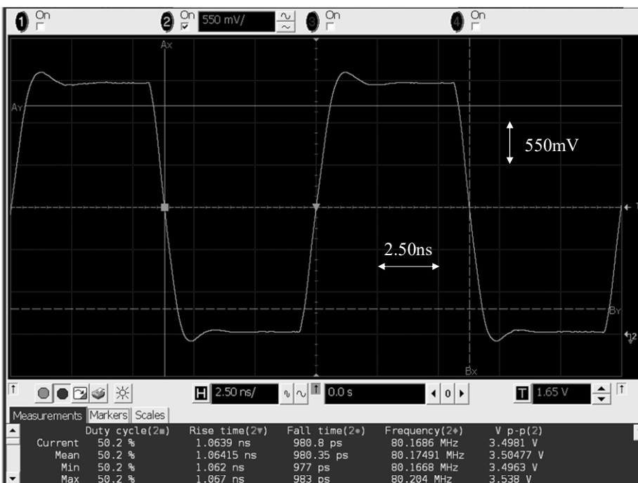
7052HxP, V_{DD}=3.3V , f_{OUT}=80MHz , C_{LOUT}=15pF , T_a=25^{\circ}C
