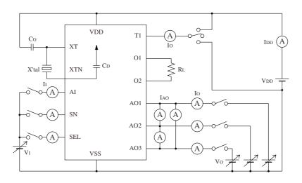
X'tal f\_0 = 32.768kHz, C\_I = 35k\Omega max, C\_L = 12.5pF, C\_0 = 1.3pF, C\_1 = 2.6pF, C\_G = 20pF, R\_L = 400\Omega or 1kΩ
