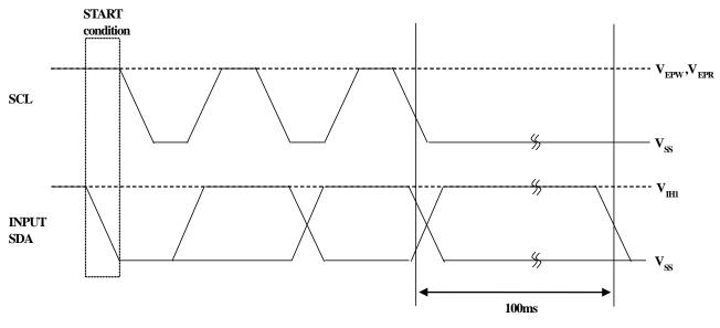
\*:When SCL isn't change from L state to H state for 100ms, the interface will be initialized automatically
