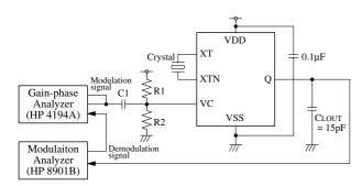
$C1=33\mu F,\,R1=R2=1M\Omega$  VC modulation signal: 100Hz to 100kHz, 0 to  $V_{DD}p\text{-}p$
