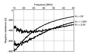
$V_{DD}$  = 3.3V, C0 = 2pF, Ta = R.T.
