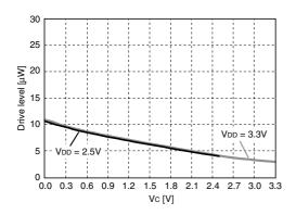
$V_{DD}$  = 2.5V, 3.3V,  $f_{OUT}$  = 27MHz, Ta = R.T.
