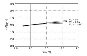
$f_{OUT}$  = 27MHz,  $\pm$  0ppm at  $V_{DD}$  = 2.5V, Ta = R.T.
