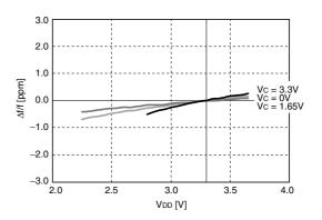
$f_{OUT}$  = 27MHz,  $\pm$  0ppm at  $V_{DD}$  = 3.3V, Ta = R.T.
