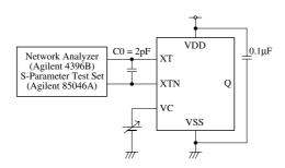
Note. "C0" value is set, concerning the actual crystal characteristics connected between XT and XTN. The data is measured with Agilent 4396B using NPC's original measurement jig. The values may vary with measurement jig and conditions.
