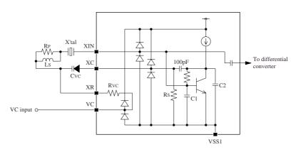
Note. R<sub>P</sub> is a damping resistor to prevent parasitic oscillation due the combined effects of the external inductor (expander coil) and varicap capacitance/internal capacitance. It is recommended that R<sub>P</sub> be connected in parallel with L<sub>S</sub>.
