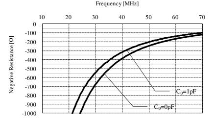
5058Hx1,  $V_{DD}$ =1.8V,  $T_a$ =25°C Measurement equipment: Agilent Impedance analyzer 4396B
