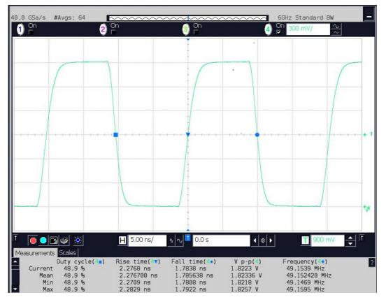
5058Hx1 version,  $V_{DD}$ =1.8V,  $f_{OUT}$ =49.15MHz,  $C_{LOUT}$ =15pF,  $T_a$ : Room temperature
