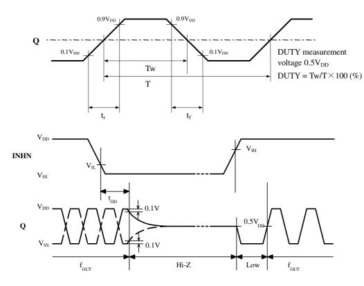
$\cdot$  When INHN goes HIGH to LOW, the Q output becomes high impedance.
