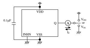
Measurement circuit 6 Parameter: R<sub>PU1</sub>, R<sub>PU2</sub>
