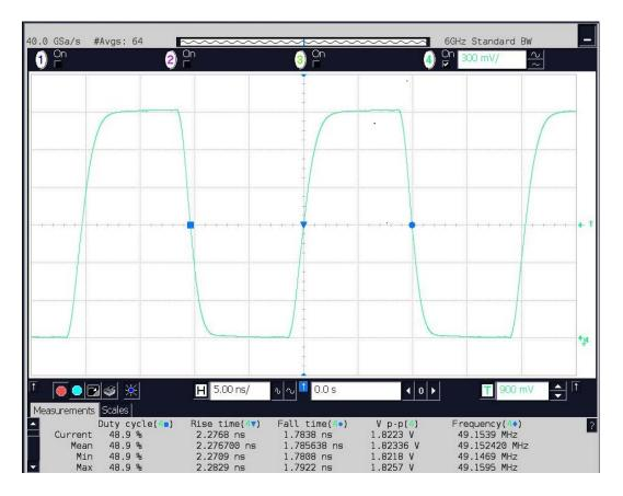
5058HA1 version,  $V_{DD}$ =1.8V,  $f_{OUI}$ =49.15MHz,  $C_{LOUI}$ =15pF,  $T_a$ : Room temperature
