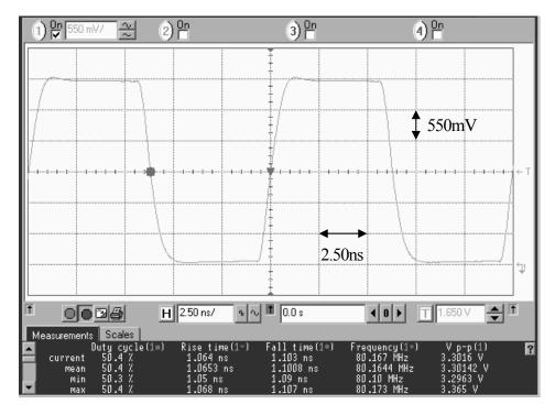
5052HxP version,  $V_{DD}$ =3.3V,  $f_{OU1}$ =80MHz,  $C_{LOU1}$ =15pF,  $T_a$ : Room temperature Measurement equipment: Oscilloscope Agilent DSO80604B
