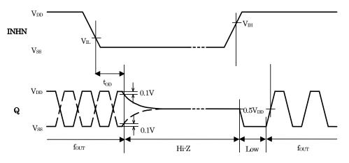
When INHN goes HIGH to LOW, the Q output becomes high impedance.
