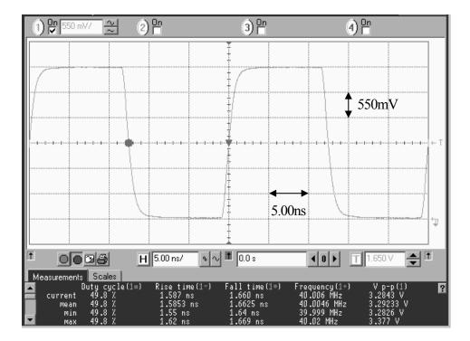
5052Hx1 version, V<sub>DD</sub>=3.3V, f<sub>OUT</sub>=40MHz, C<sub>LOUT</sub>=15pF, T<sub>a</sub>: Room temperature
