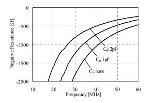
5052Hx1,  $V_{DD}$ =3.3V,  $T_a$ =25°C Measurement equipment: Agilent Impedance analyzer 4396B
