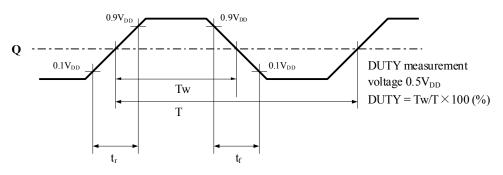
Figure 1. Output switching waveform
