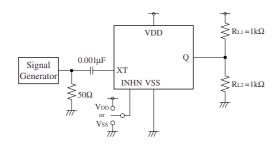
XT input signal: 1Vp-p, sine wave
