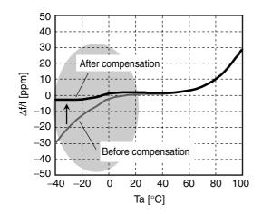
Figure 5. Low-temperature characteristics compensation
