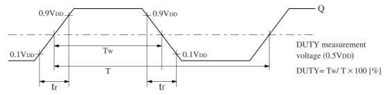
Figure 1. Output switching waveform
