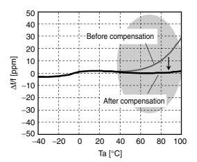
Figure 6. High-temperature characteristics compensation
