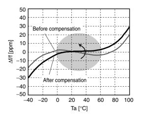
Figure 4. Temperature rotation compensation
