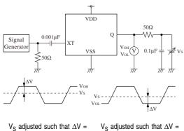
$v_{\rm S}$  adjusted such that  $\Delta v$  50  $\times$   $I_{\rm OH}.$
