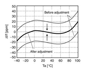
Figure 3. Center frequency adjustment
