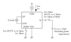
Note: The AC characteristics are observed using an oscilloscope on pin Q.
