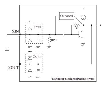
The 5037A1/B $\times$ /C $\times$ /D $\times$ (T)/E $\times$  oscillator circuit has a C0 cancel circuit built-in to improve the oscillator margin. If power is applied when there is an open circuit between XIN and XOUT, self oscillation may occur, which is not abnormal. Users should confirm that the oscillator operates normally when a crystal unit is connected.
