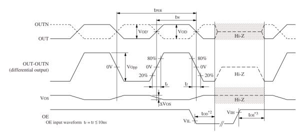
$DUTY = t_W / t_{PER} \times 100$  (%) @ crossing point  $\Delta V_{OD} = |V_{OD}' - V_{OD}|$
