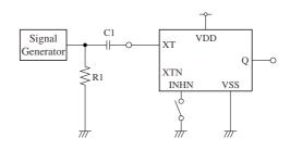
1Vp-p, 10MHz sine wave input signal
