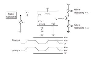
2Vp-p, 10MHz sine wave input signal
