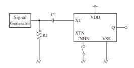
2Vp-p, 10MHz sine wave input signal
