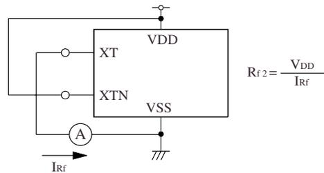
$$R_{f2} = \frac{V_{DD}}{I_{Rf}}$$
