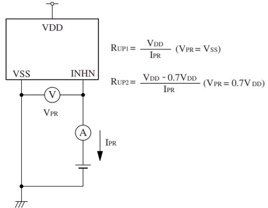
$$R_{UP1} = \frac{V_{DD}}{I_{PR}} \quad (V_{PR} = V_{SS})$$
