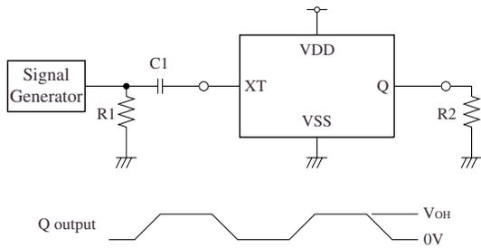
2.5V<sub>P-P</sub>, 10MHz sine wave input signal
