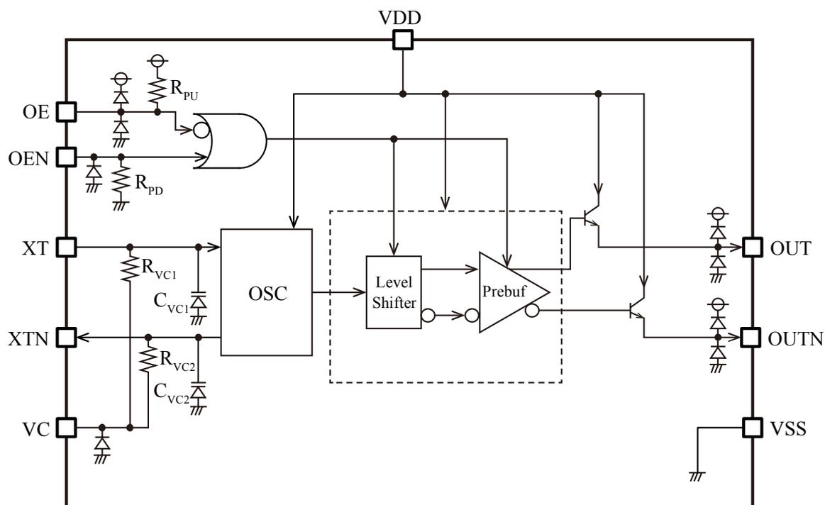
The CF5420/WF5420 incorporated standard PECL output schemes, which are un-terminated emitters.
