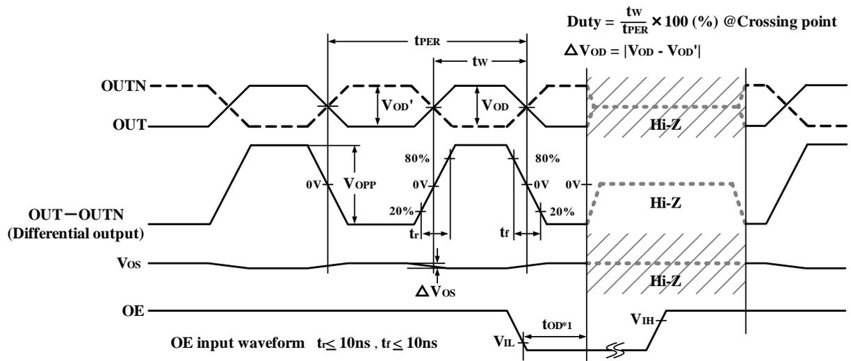
\*1. The OUT/OUTN output goes high impedance after the OE is fallen and then the output disable time “ $t_{OD}$ ” has elapsed.
