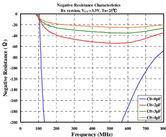
Characteristics are measured with a capacitance C0, representing the resonator equivalent circuit C0 capacitance, connected between the XIN and XOUT pins. Measurement are performed with Agilent 4396B, 85046A using the NPC test jig. Characteristics may vary with measurement jig and measurement conditions.
