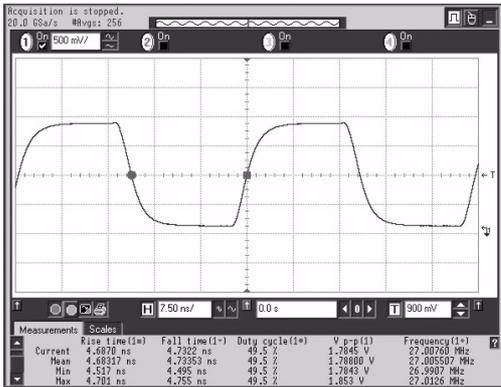
$V_{DD} = 1.8V, f_{OUT} = 27MHz, V_C = 0.5V_{DD},$
