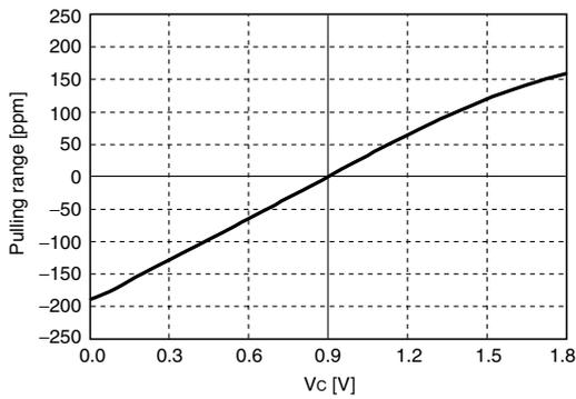
$V_{DD} = 1.8\text{V}$ ,  $f_{OUT} = 27\text{MHz}$ ,  $T_a = \text{R.T.}$
