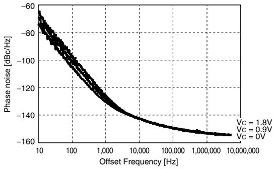
$V_{DD} = 1.8V, f_{OUT} = 27MHz, T_a = R.T.$
