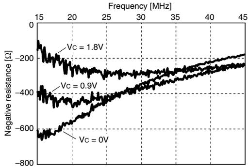
$V_{DD} = 1.8V, C_0 = 2pF, T_a = R.T.$
