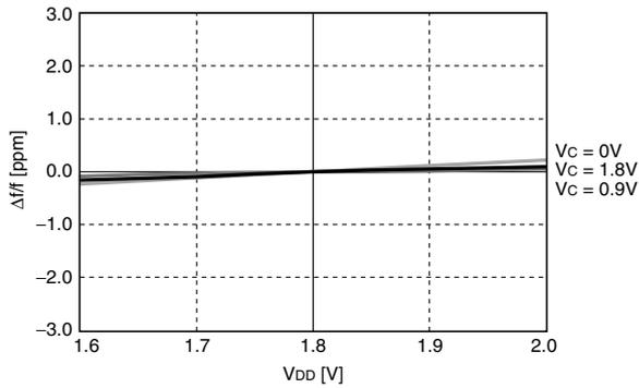
$f_{OUT} = 27MHz, \pm 0ppm \text{ at } V_{DD} = 1.8V, T_a = R.T.$
