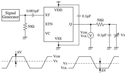
$V_S$  adjusted such that  $\Delta V = 50 \times I_{OH}$ .
