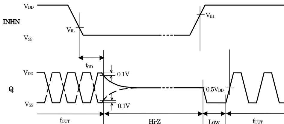
When INHN goes HIGH to LOW, the Q output becomes high impedance.
