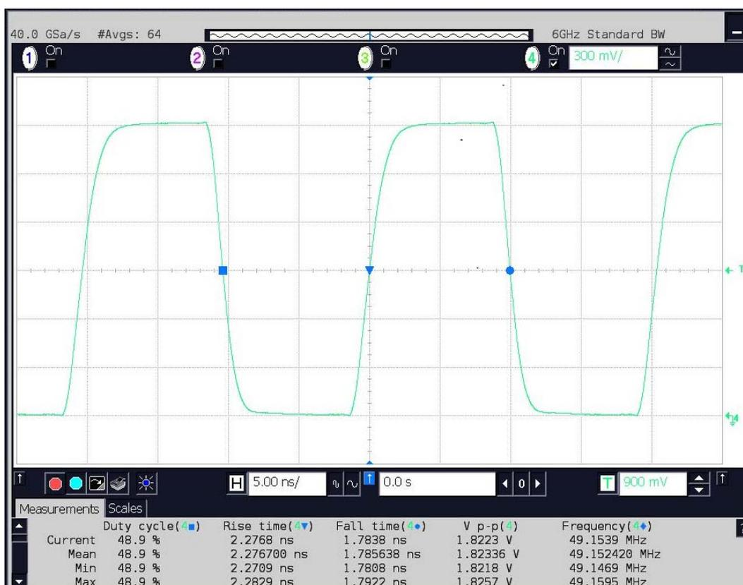
5058HA1 version,  $V_{DD}=1.8V$ ,  $f_{OUT}=49.15MHz$ ,  $C_{LOUT}=15pF$ ,  $T_a$ : Room temperature
