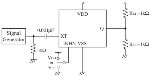
XT input signal: 1Vp-p, sine wave
