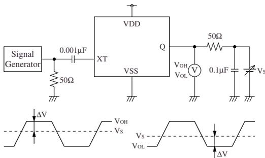
$V_S$  adjusted such that  $\Delta V = 50 \times I_{OH}$ .
