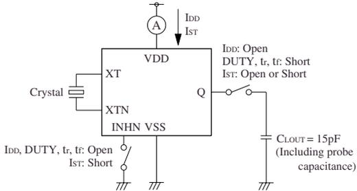
Note: The AC characteristics are observed using an oscilloscope on pin Q.
