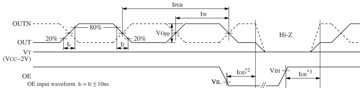
\*2. The OUT/OUTN output goes high impedance after the OE is fallen and then the output disable time " $t_{OD}$ " has elapsed. The output signal is pulled down to  $V_T$  (terminated voltage) by load resistance.
