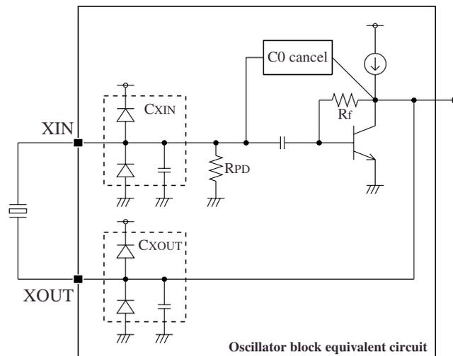
The 5036G×/A×/B×/C×/D×(T)/E× oscillator circuit has a C<sub>0</sub> cancel circuit built-in to improve the oscillator margin. If power is applied when there is an open circuit between XIN and XOUT, self oscillation may occur, which is not abnormal. Users should confirm that the oscillator operates normally when a crystal unit is connected.
