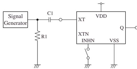
2Vp-p, 10MHz sine wave input signal
