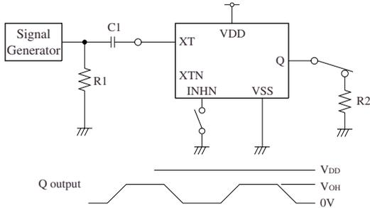
2Vp-p, 10MHz sine wave input signal
