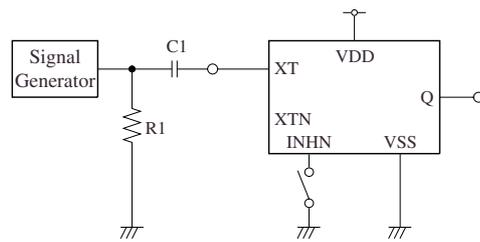
2Vp-p, 10MHz sine wave input signal
