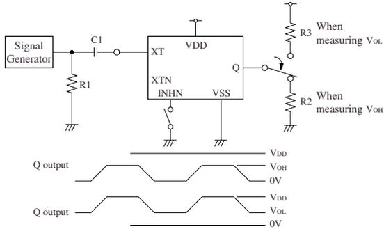
2Vp-p, 10MHz sine wave input signal
